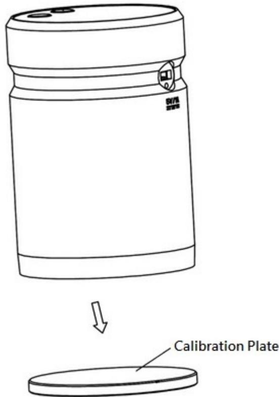
**⚠** It is recommended to conduct calibration every six months. This product has a self-adaptability design. Frequent calibration does not help to increase accuracy.
