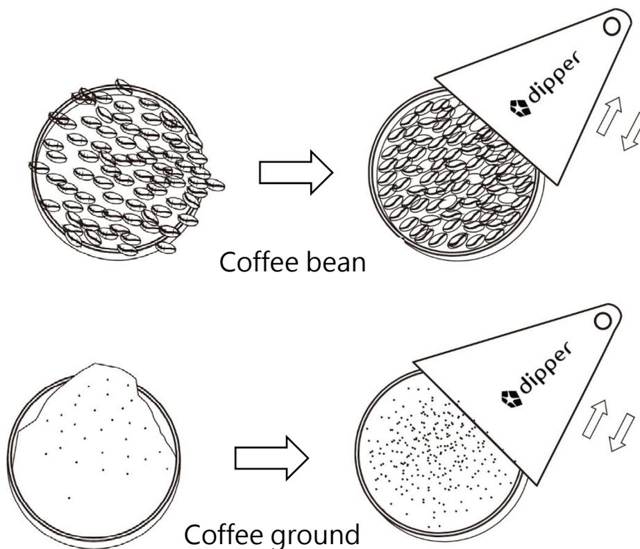
The degree of coffee grinding will also affect the measurement result. The SCA cupping standards requires 70 to 75% of ground must pass through 20 mesh sieve. The ground is then flattened to fill the sample cup. Make sure
