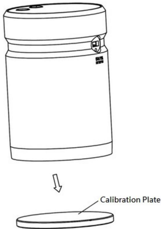
**⚠** It is recommended to conduct calibration every 3 to 6 months. This product has a self-adaptability design. Frequent calibration does not help to increase accuracy.
